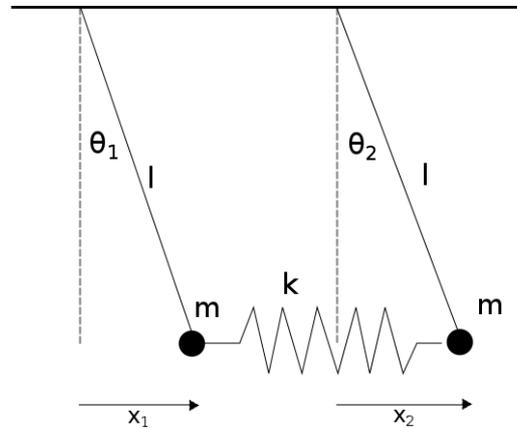
Figure 3.2: Two identical pendula joined by a spring
